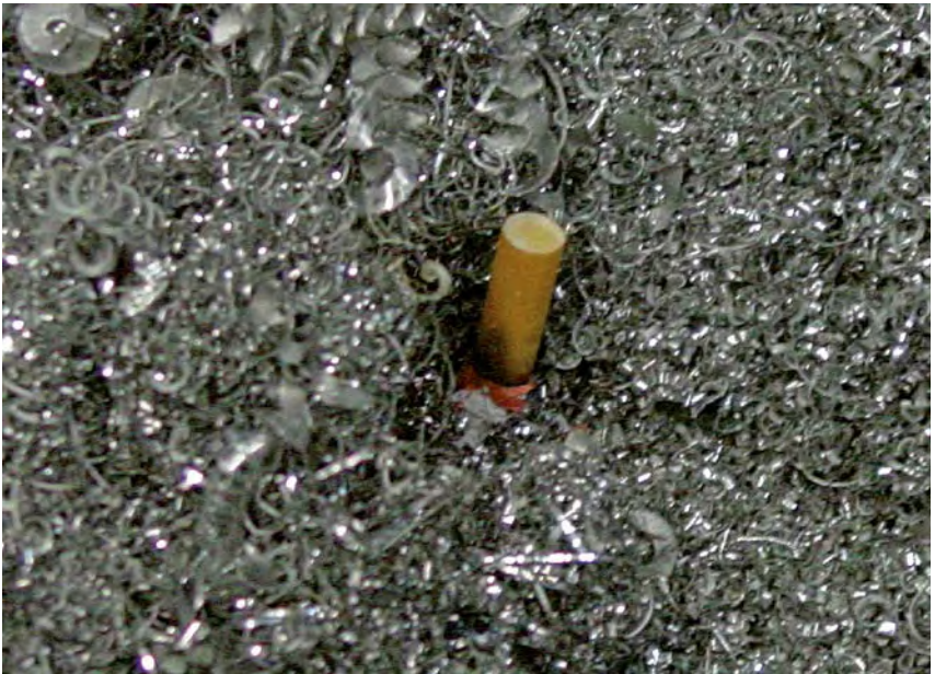
Figure 56 Source of ignition in the chip container
