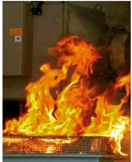
Figure 44 After-Fire subsequent to extinguishing
