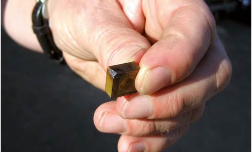
Figure 19 Worn indexable cutting insert
