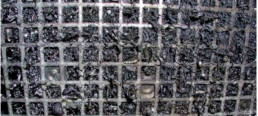
Figure 35 Clogged chip grating
