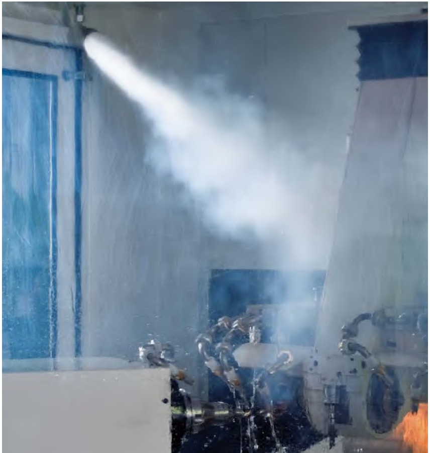
Figure 48 Extinguishing after fire detection
