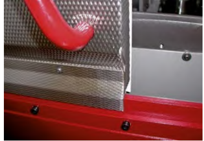
Figure 26 Detail of a sliding door with additional labyrinth for machining with neat oil
