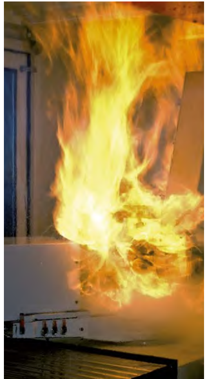
Figure 47 MWF ignition during grinding with subsequent fire
