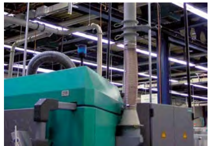
Figure 37 Connecting piece for vibration isolation: vertical, earthed
