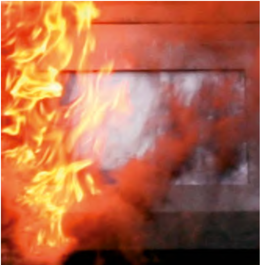
Figure 23 Flame ejection from a door labyrinth
