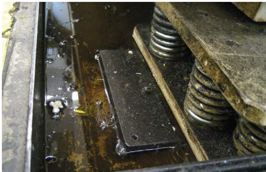
Figure 22 Machine tool in "oil bath"
