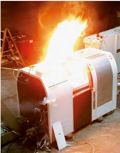
Figure 43 Flame ejection from a pressure relief valve
