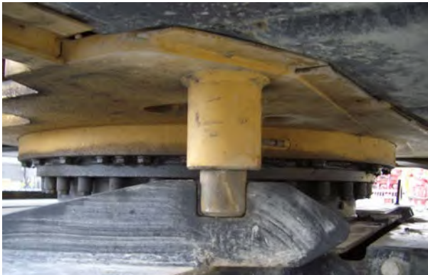
Fig. 40 Swivel lock on a hydraulic excavator in locked position
