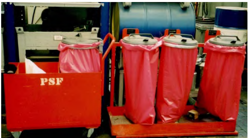
Fig. 7 Trolley for transporting oil binders
