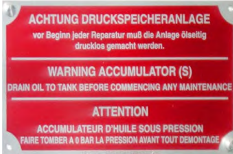
Fig. 21 Warning note on accumulator system
