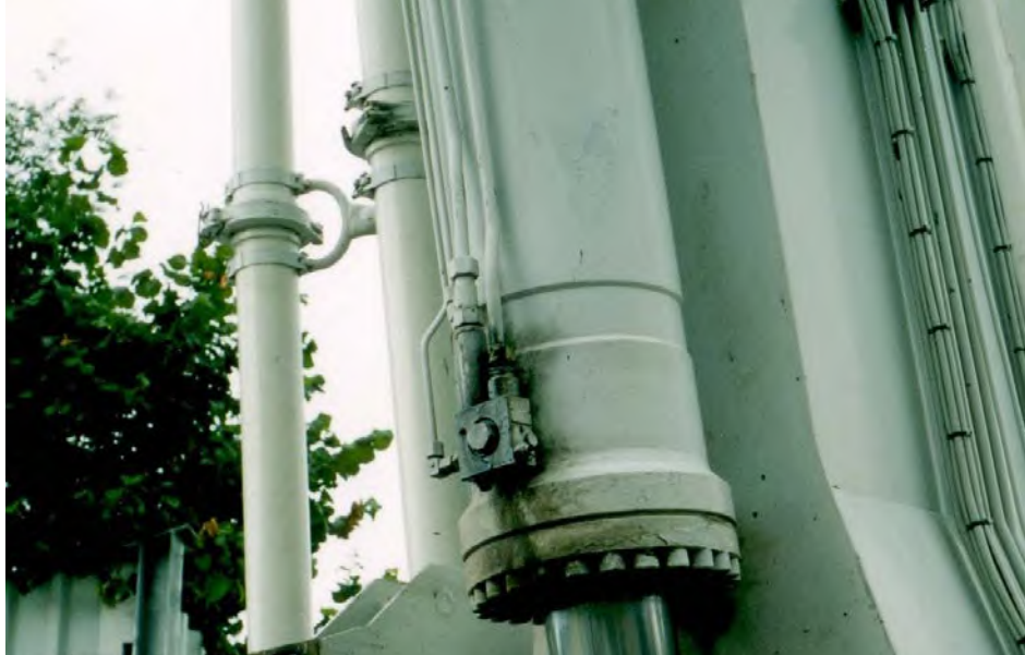
Fig. 18 Hydraulic cylinder with pilot-operated check valve
