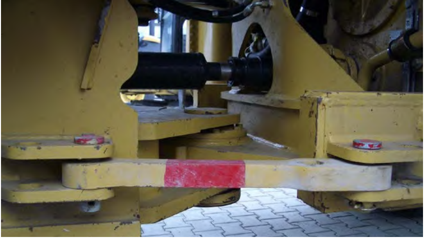
Fig. 30 Installed articulated steering lock
