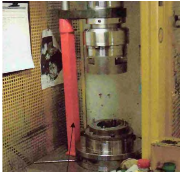
Fig. 28 Slide support on a hydraulic press
