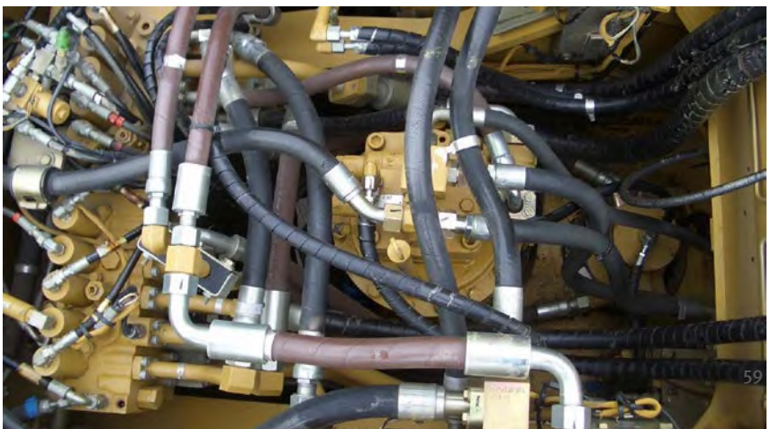
Fig. 32 Hose assemblies on a mobile hydraulic system
