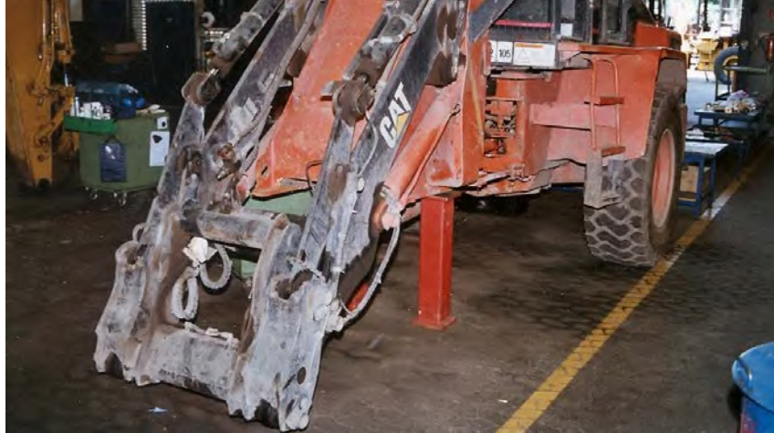
Fig. 33 Support frame when working on wheel-type loaders
