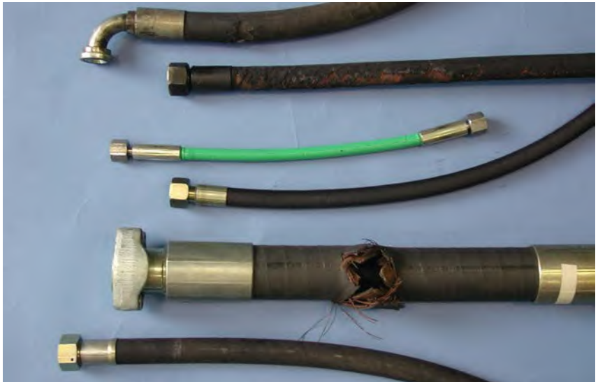
Fig. 16 Examples of failed hydraulic hose assemblies
