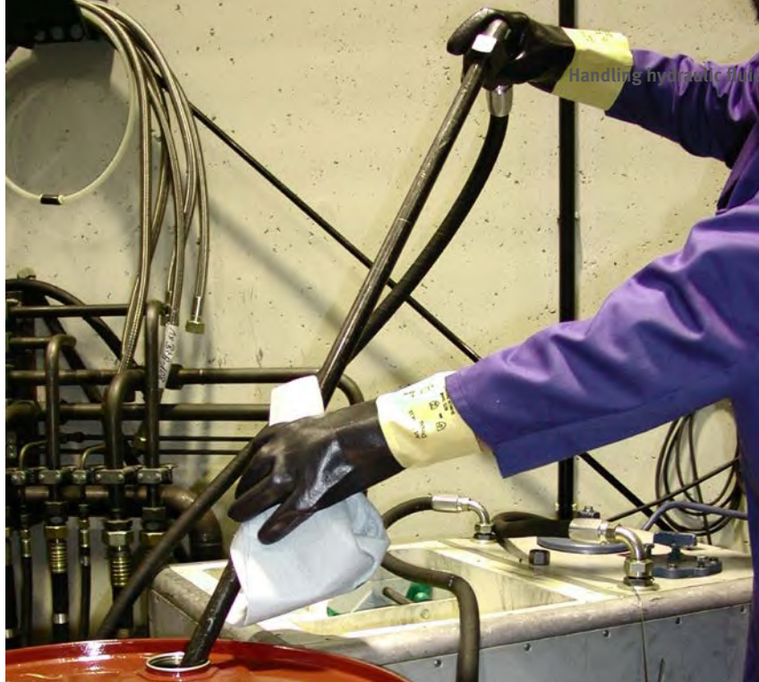
Fig. 5 Personal protective equipment for oil change
