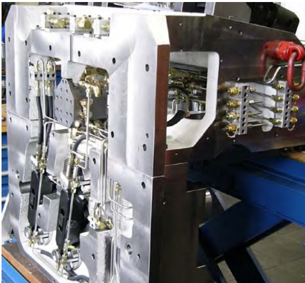
Fig. 27 Complex clamping module of a transfer line
