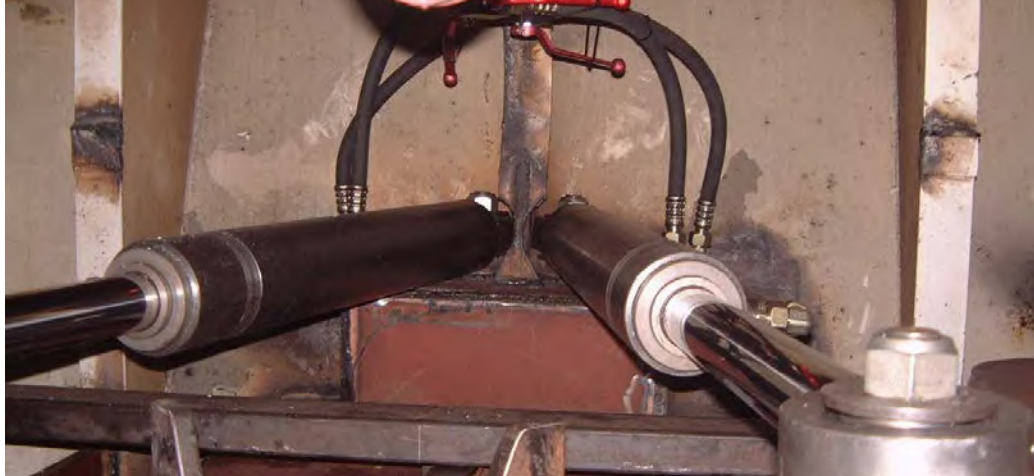
Fig. 43 Risks of pinching on a rudder system
