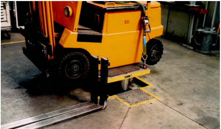
Fig. 35 Lifting forks removed for working on the hydraulic system of a fork-lift truck
