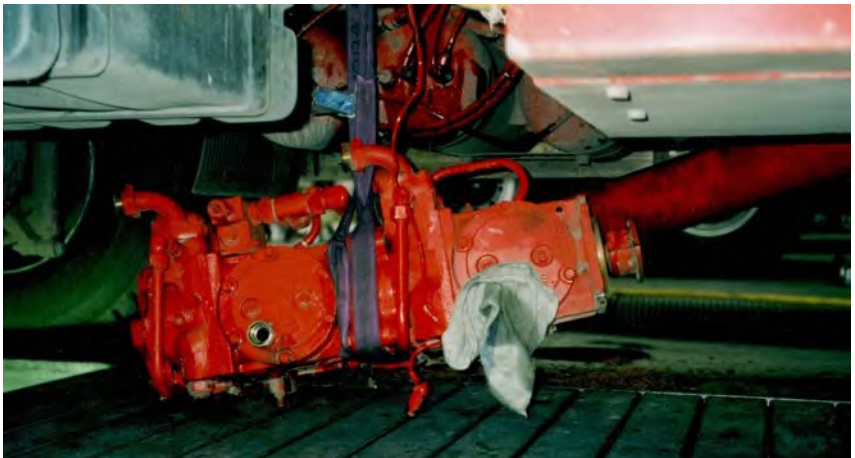
Fig. 39 Vehicle main pump on a load lifting device
