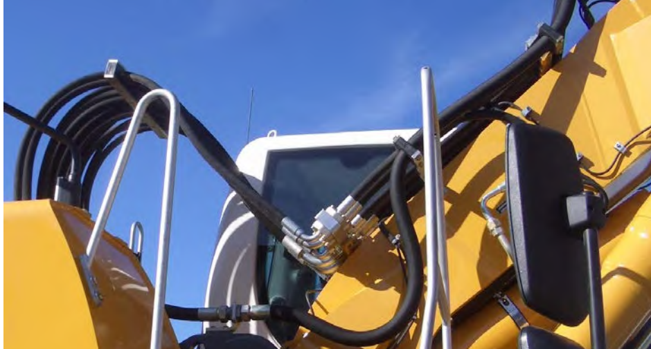
Fig. 12 Hydraulic hose assemblies on an excavator
