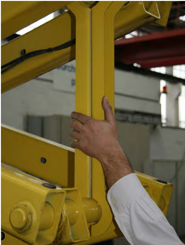
Fig. 29 Installed maintenance support on hydraulic scissors lift
