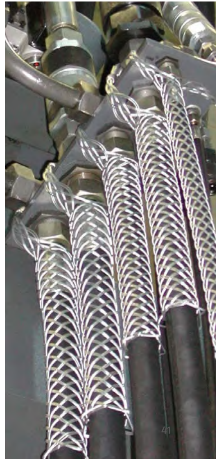
Fig. 17 Stripping protection on hose assemblies
