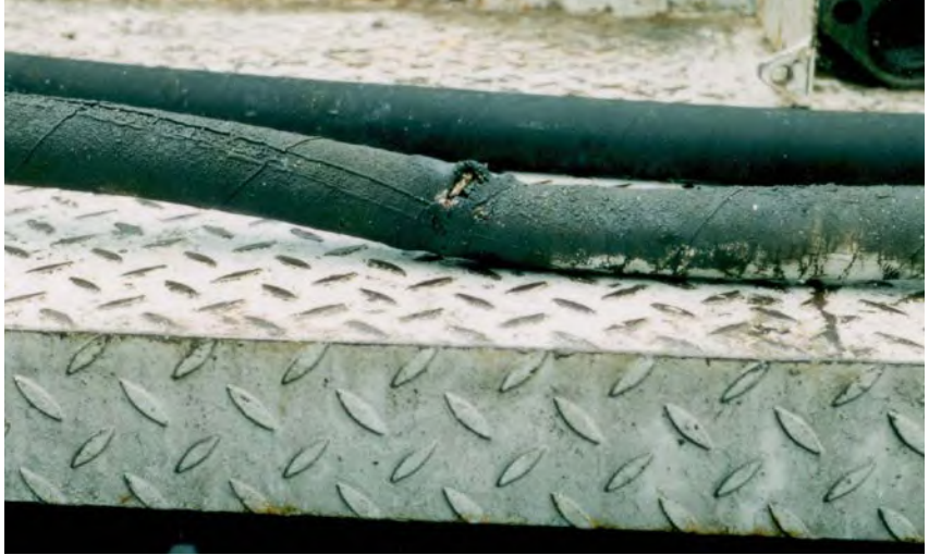
Fig. 2 Bursted hydraulic hose assembly
