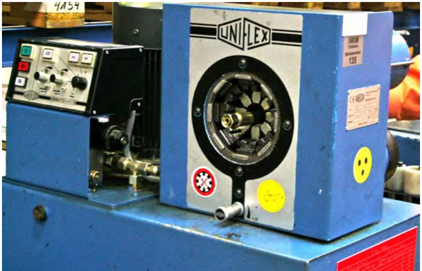
Fig. 14 Device for pressing hose fittings
