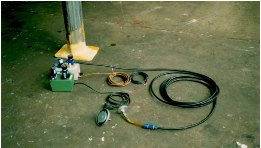
Fig. 8 Vacuum pumps for mobile hydraulic tank in 24 VDC and 230 VAC design
