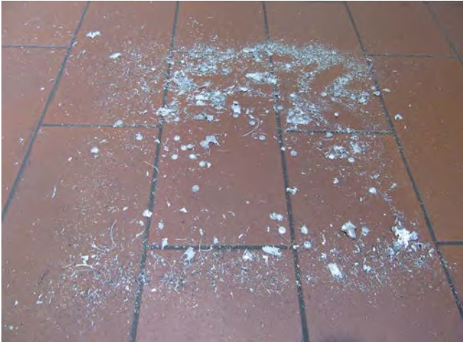
Figure 2 Residues from dry processing (magnesium dusts and chips)
