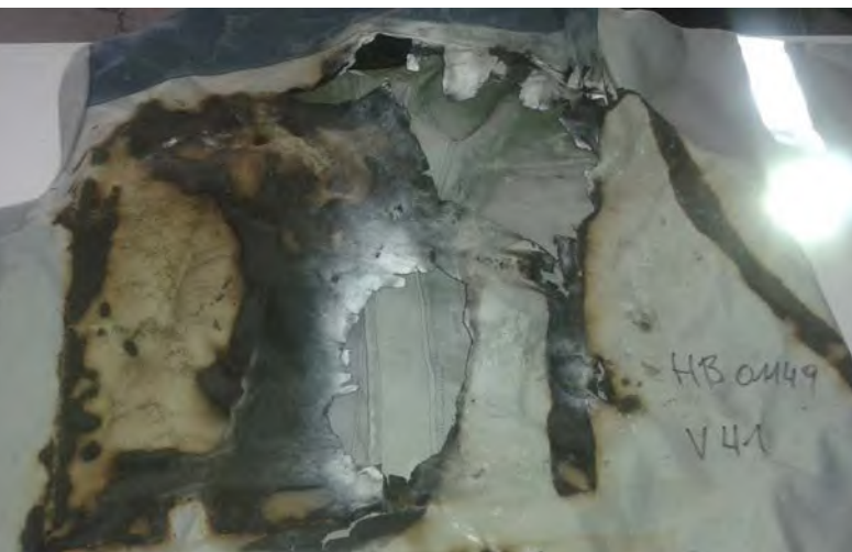
Figure 29 Burnt unsuitable protective clothing
