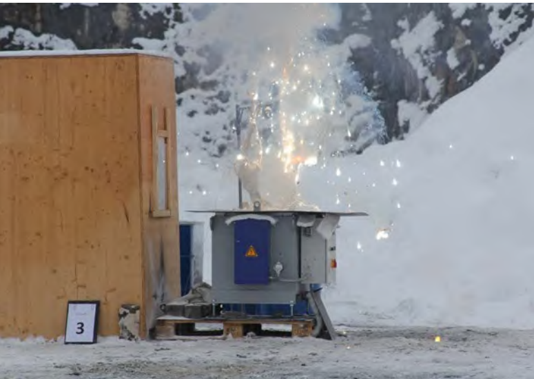
Figure 13 Fire of molten magnesium
