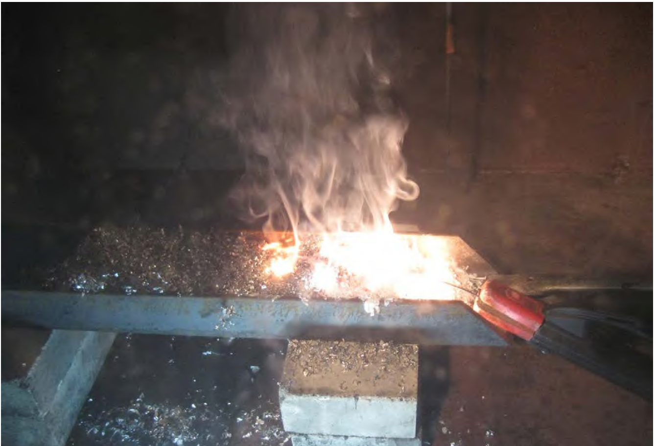
Figure 1 Burning magnesium residues
