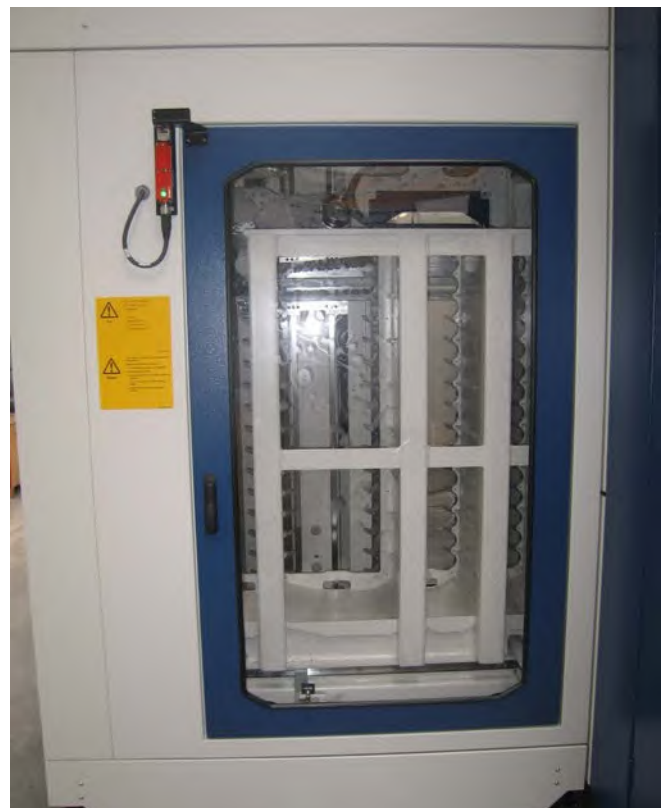
Figure 12 Interlocking guard with guard locking/position switch with emergency unlocking at the protection door magazine maintenance
