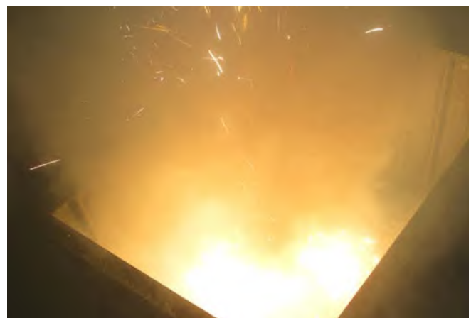
Figure 4 Burning magnesium in the chip container
