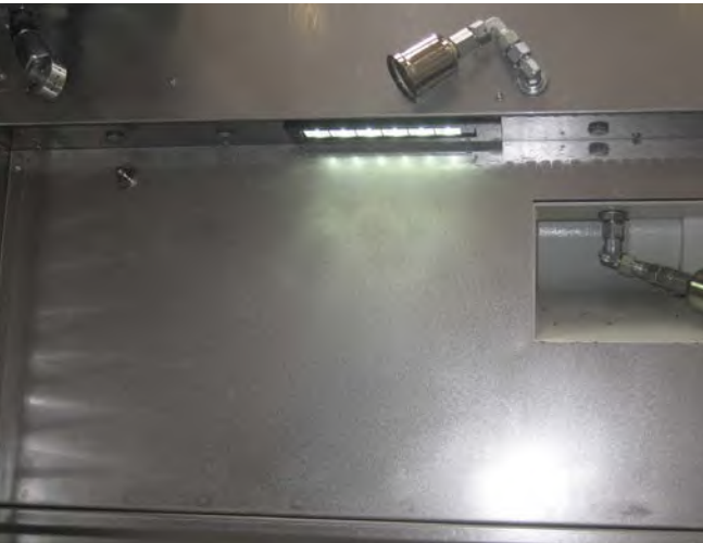
Figure 11 Extinguishing nozzle and heat detector/temperature sensor in the interior of the machine
