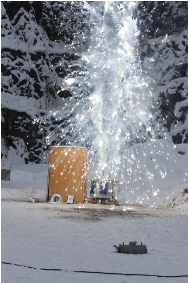
Figure 14 Ejection of molten metal on contact with water, approx. 50 ml
