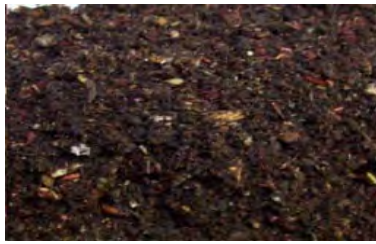
Figure 1.7: Hazardous waste – impregnated sawdust
