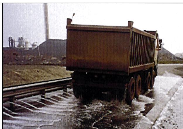
Figure 4.32: A pool of water in combination with running water for the tyres' running surface [134, Corus, 1995]
