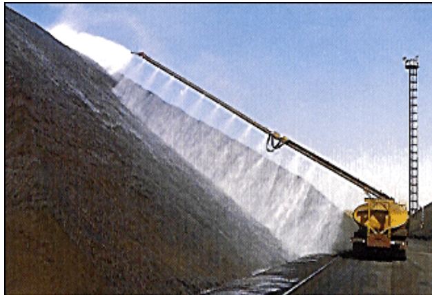
Figure 4.20: Uniform spraying is extremely important for the formation of a good crust [134, Corus, 1995]
