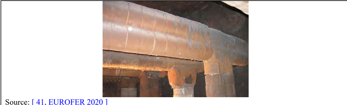
Figure 2.86: Double-pipes skid design for reheating furnaces
