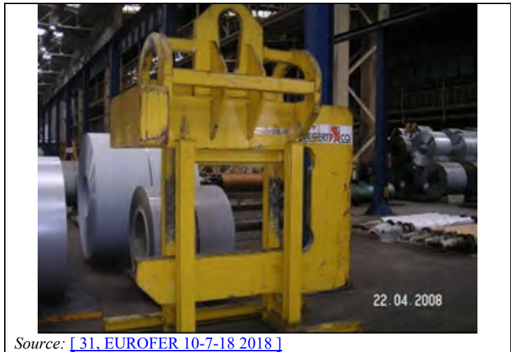
Figure 8.5: C-hook magnet for hoisting of coils
