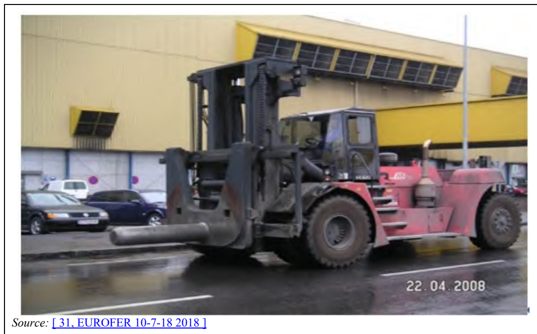
Figure 8.6: Piler with mandrels for coil manipulation and transport
