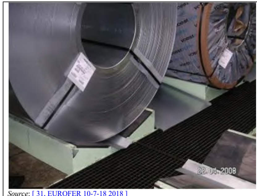
Figure 8.2: Coil support lined with rubber corresponding to the coil geometry
