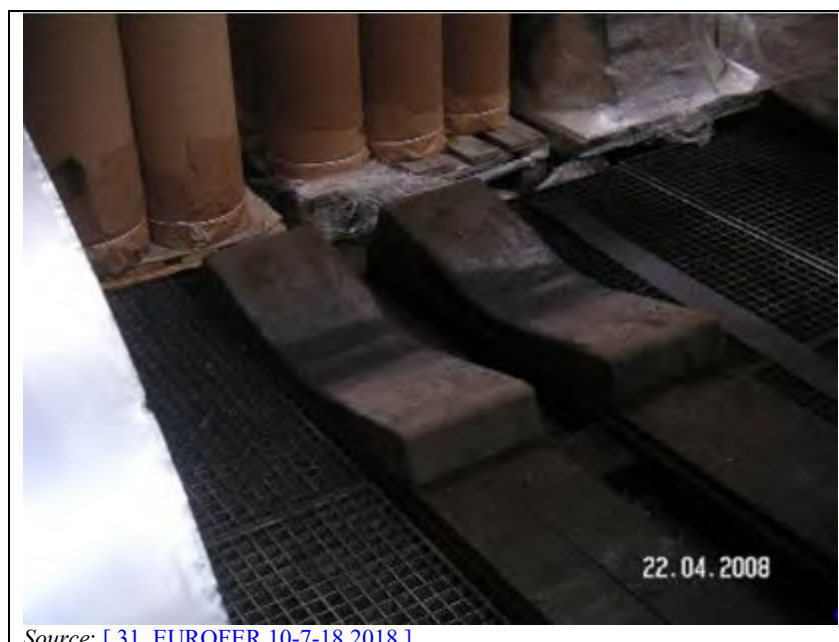
Figure 8.3: Coil support with oil drip trays
