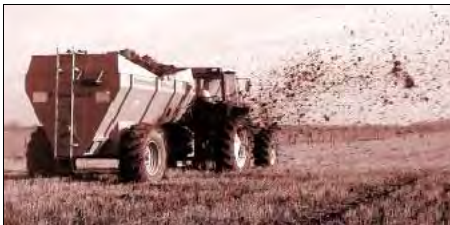
Figure 2.46: Example of a dual purpose spreader [51, MAFF, 1999]
