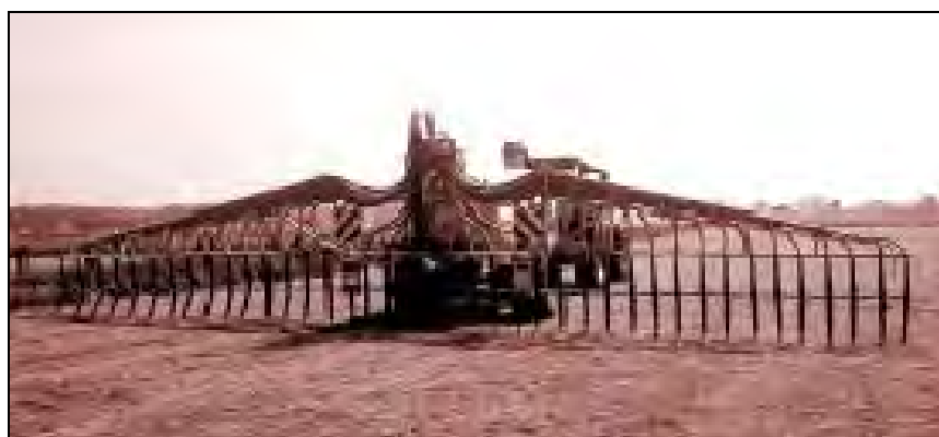
Figure 2.40: Example of a band spreader fitted with rotary distributor to improve lateral distribution [51, MAFF, 1999]
