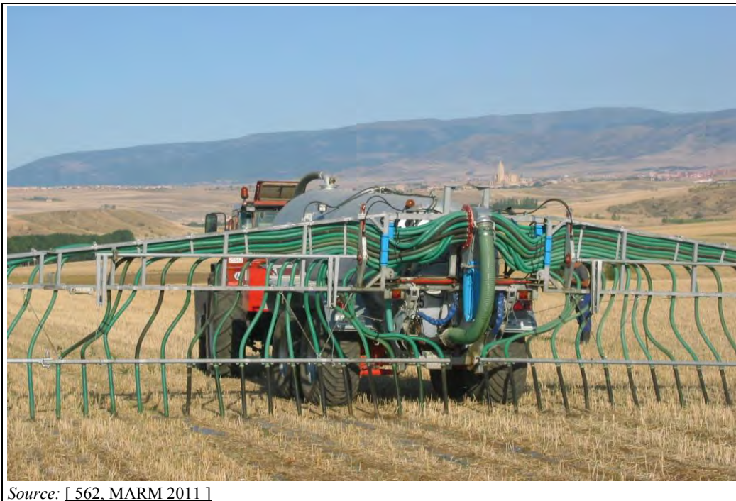
Figure 2.37: Example of a band spreader fitted with rotary distributor to improve lateral distribution
