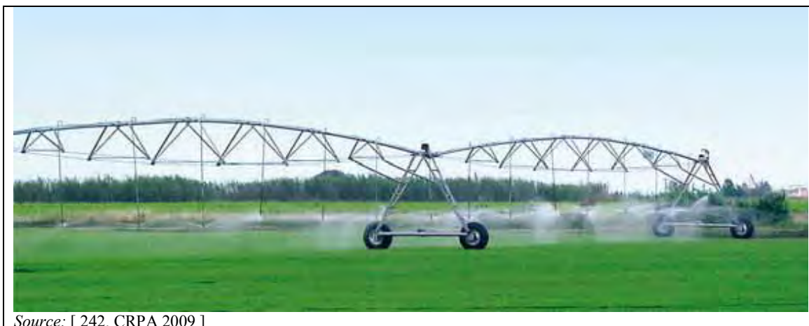
Figure 4.95: Irrigation boom fitted with hanging nozzles to spray the water-slurry mixture close to the soil surface
