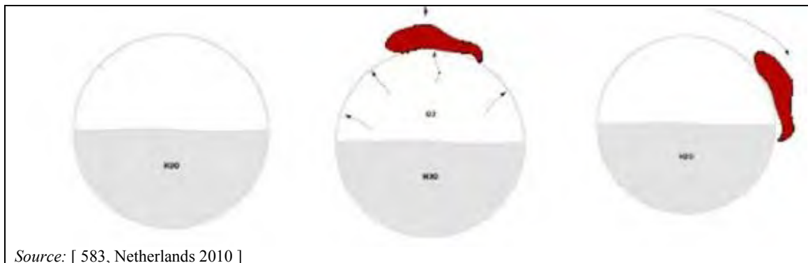
Figure 4.69: Schematic representation of the functioning principle of floating balls
