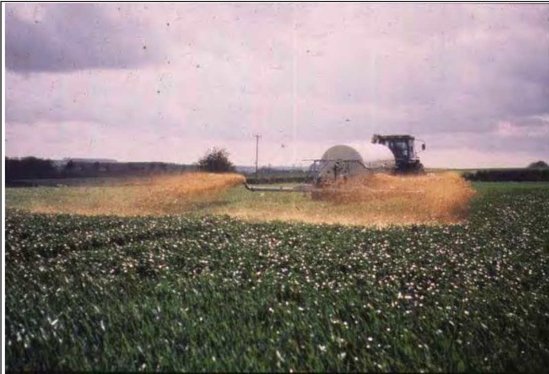
Figure 2.34: Example of a broadcast technique with low trajectory and low pressure
