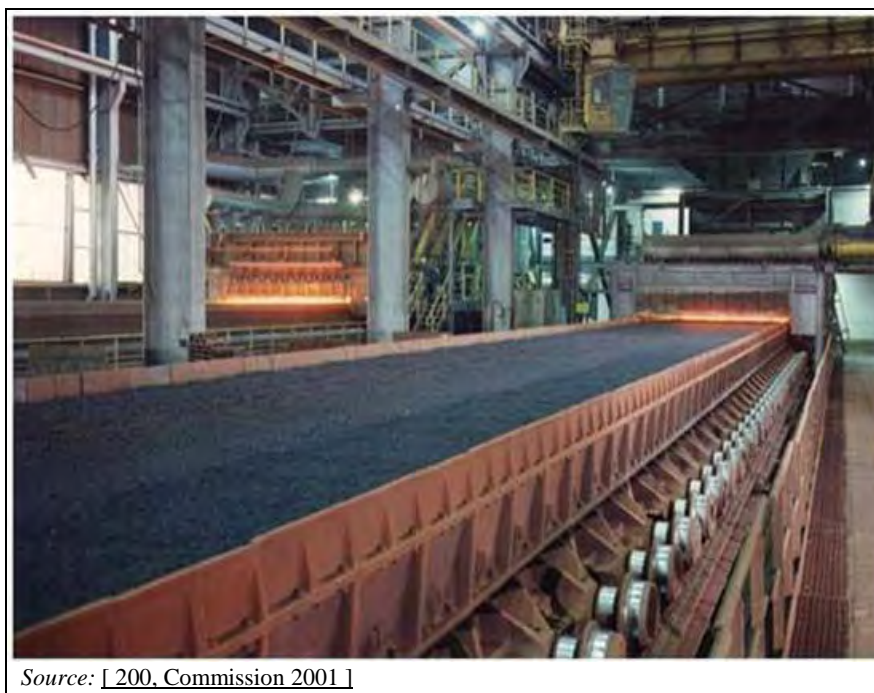
Figure 3.1: Photograph of a sinter strand with the charging facility (drums or chutes) and the ignition canopy at the starting end
