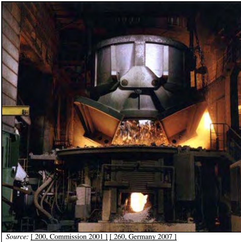
Figure 8.2: Electric arc furnace charging
