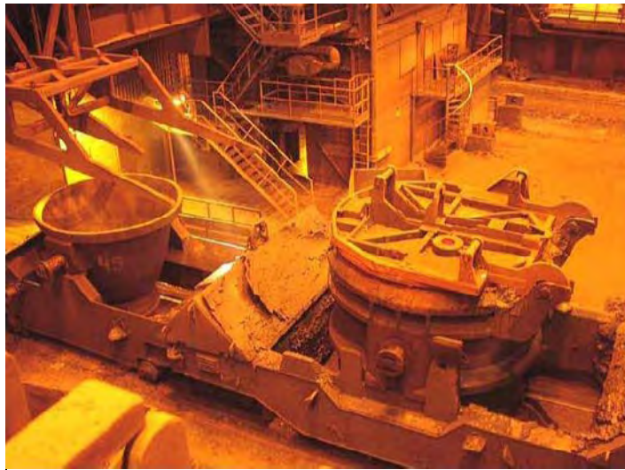
Figure 7.24: Automatic ladle lid system
