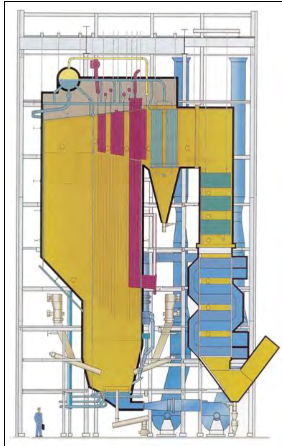
Figure 4.13: CFBC boiler for burning low-sulphur coal [83, Foster Wheeler, 1995]
