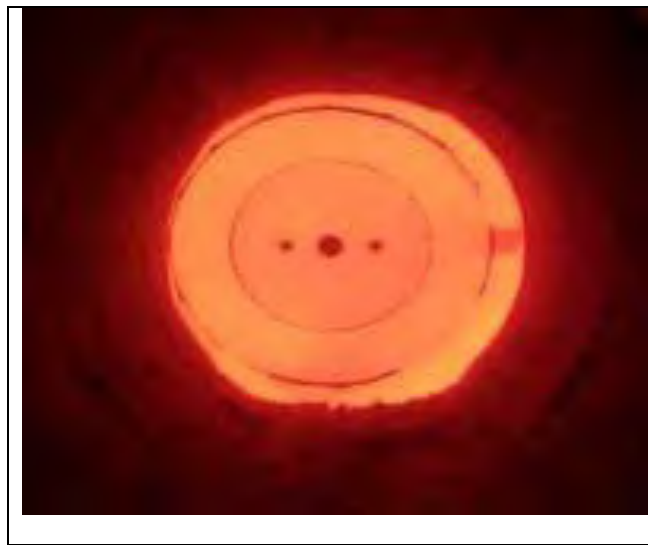
Figure 11.7: Typical picture of combustion obtained with a flameless burner
