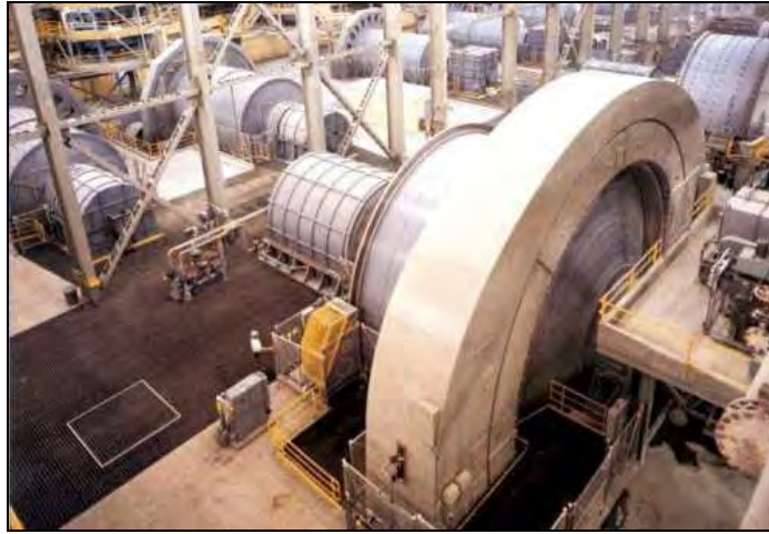
Figure 2.5: Grinding circuit with AG mills (primary grinding, right side) and ball mills (secondary grinding, left side)
