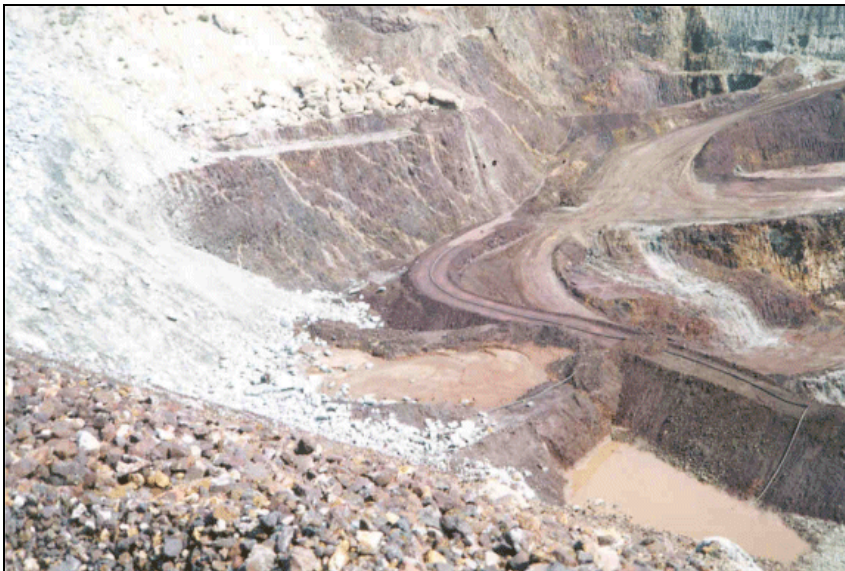
Figure 3.48: Dewatering of barytes tailings in the pit [110, IGME, 2002]
