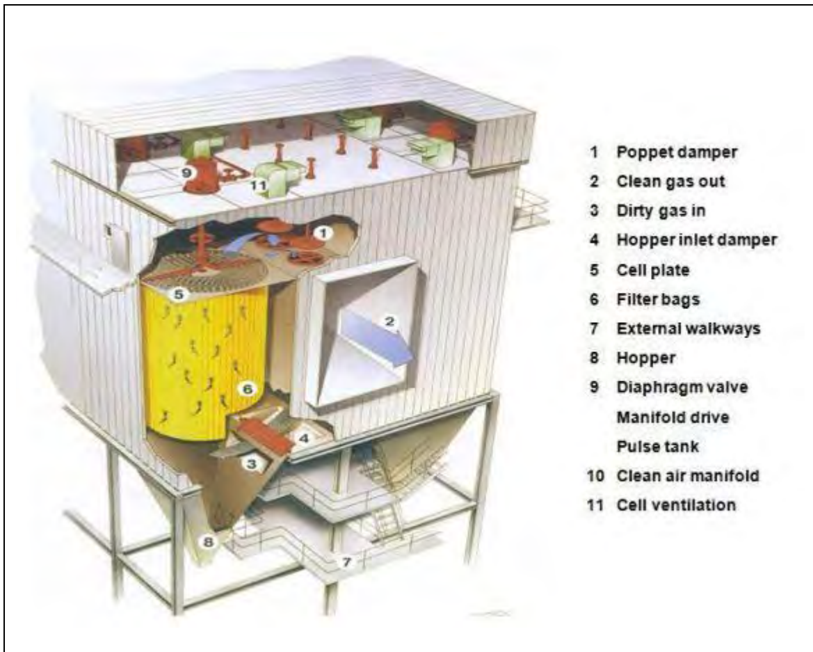
Figure 2.28: Low-pressure air pulsing cleaning system
