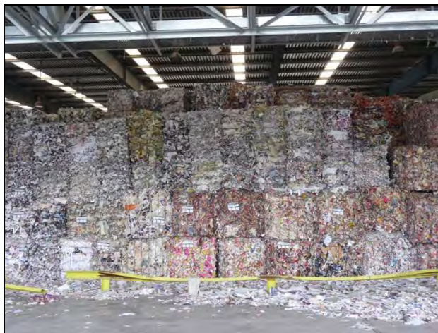
Figure 6.31: Storage of paper for recycling in bales under a roof
