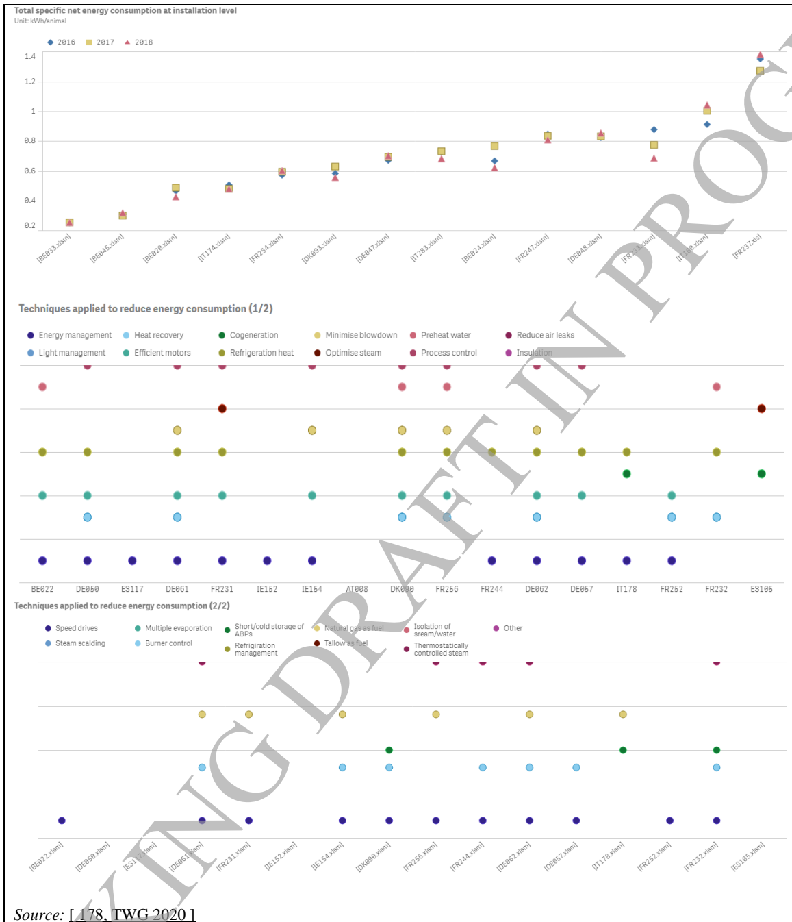
Figure 3.66: Specific net energy consumption (kWh/animal) and applied techniques to reduce energy consumption in chicken slaughterhouses (installation level)
