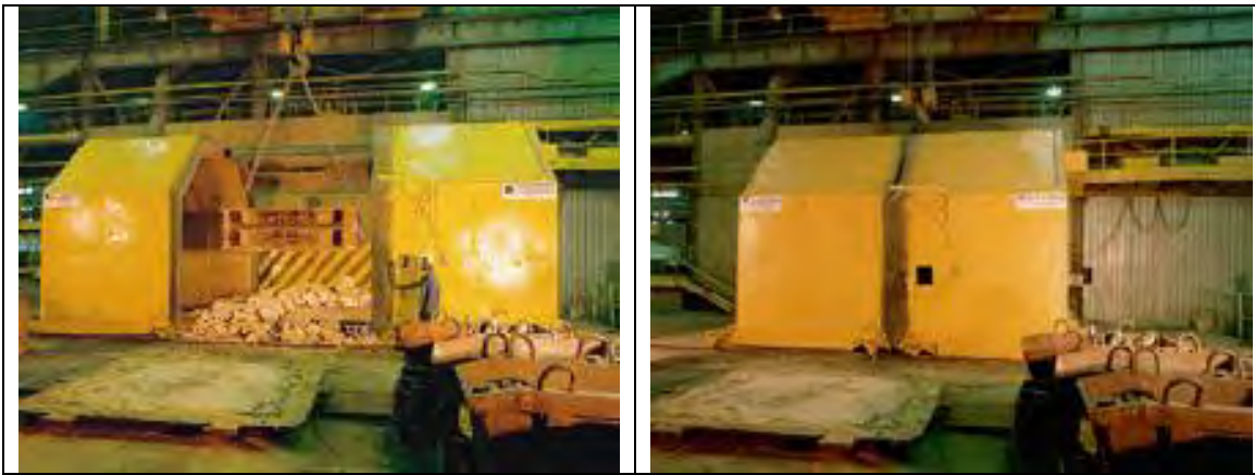
Figure 4.17: Doghouse cover for a shake-out grate, for large-size batch castings [209, Metalodlew s.a., 2003]
