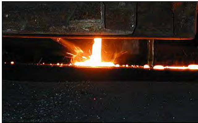
Figure 2.24: Inoculation during pouring [237, HUT, 2003]
