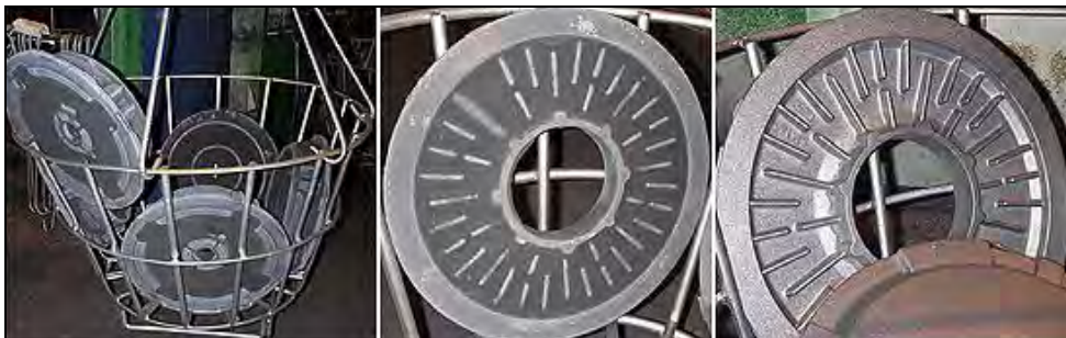
Figure 2.50: Castings before (l., m.) and after (r.) sand removal by blasting [237, HUT, 2003]
