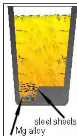
Figure 2.23: The sandwich method for nodularisation [237, HUT, 2003]
