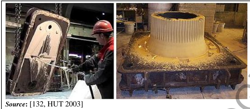
Figure 2.38: Flow coating with alcohol-based coating, followed by firing or drying
