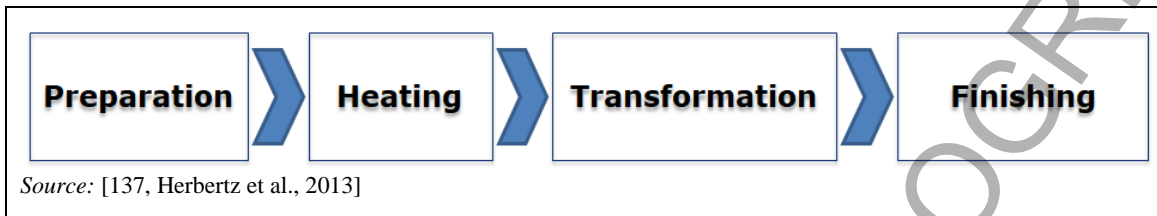
Figure 1.4: Basic process chain of forging processes
