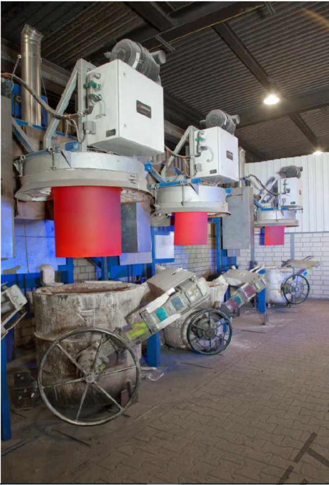
Figure 3.6: Ladle preheating using porous burners
