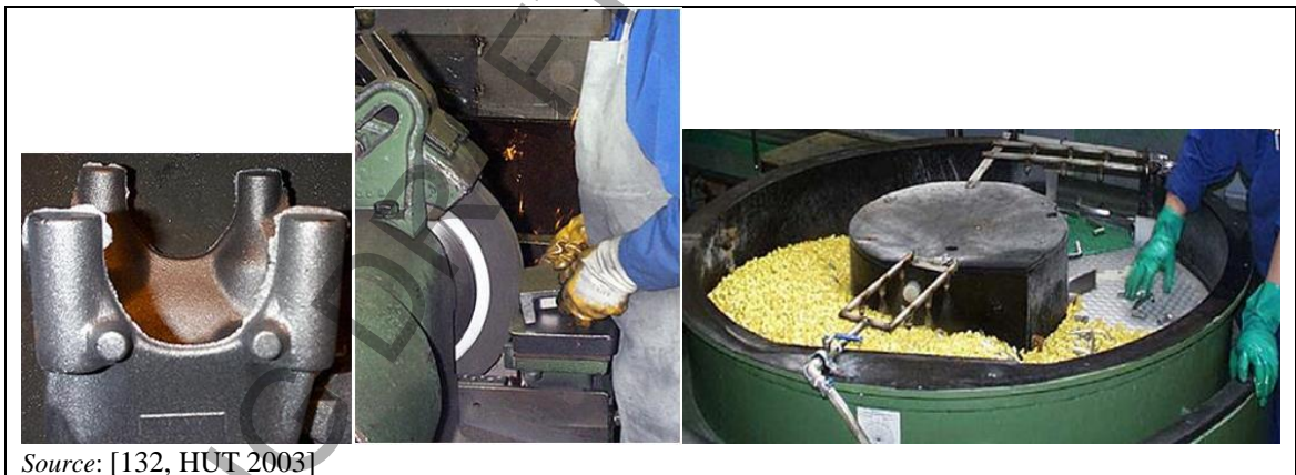
Figure 2.55: Burrs (L) and their removal using a grinding stone (C) and slide grinding (R)
