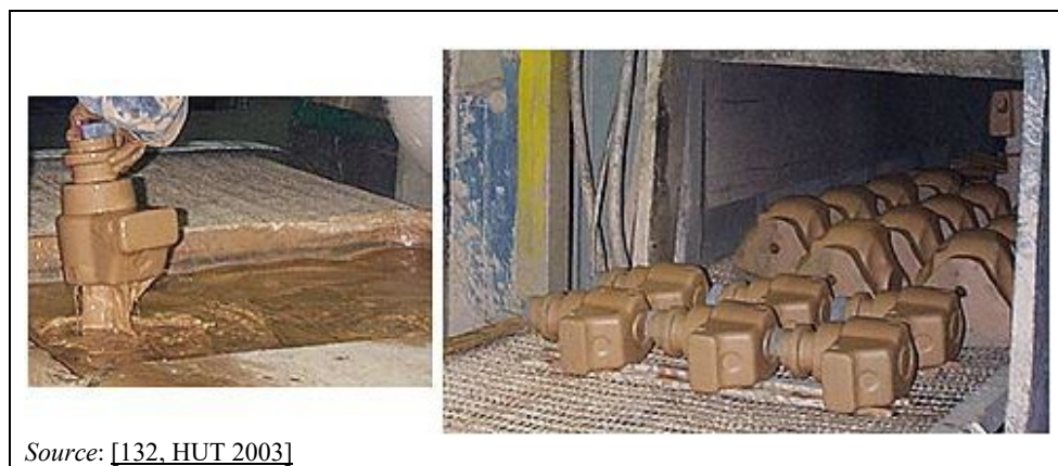
Figure 2.38: Dip-coating with water-based coatings, followed by drying in a hot-air furnace
