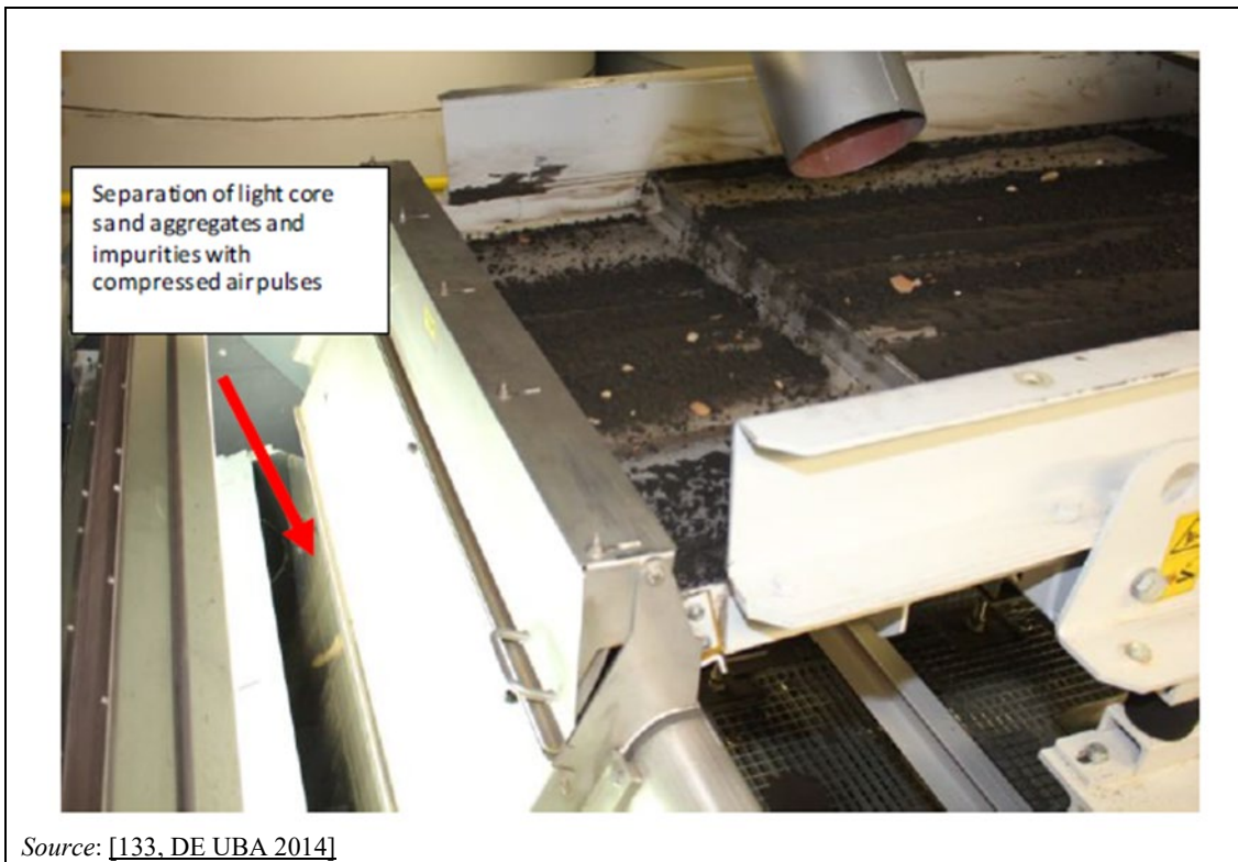
Figure 3.22: Device for optical detection and separation of impurities from green sand
