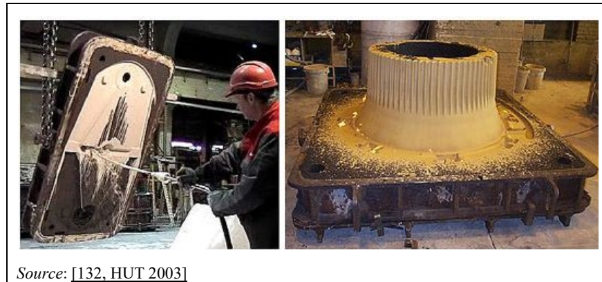
Figure 2.37: Flow coating with alcohol-based coating, followed by firing or drying
