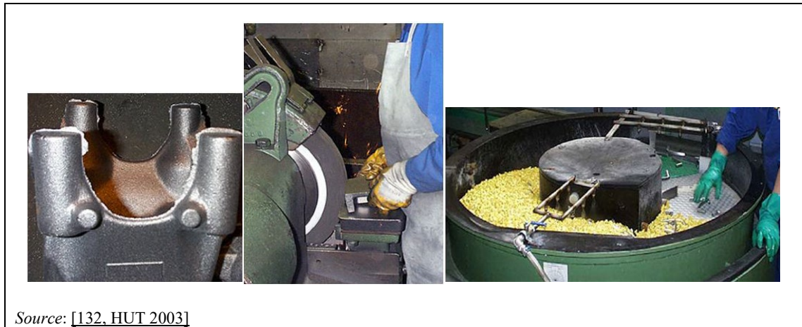
Figure 2.55: Burrs (L) and their removal using a grinding stone (C) and slide grinding (R)
