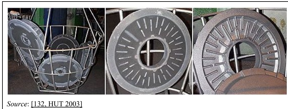
Figure 2.54: Castings before (L, C) and after (R) sand removal by blasting
