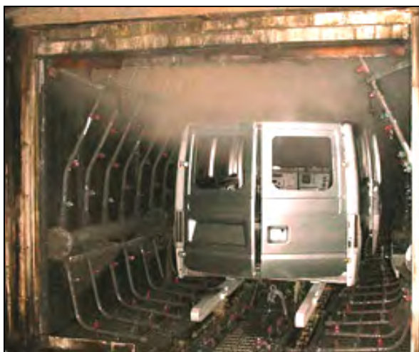
Figure 2.4: Automotive body undergoing spray pre-treatment [ACEA]
