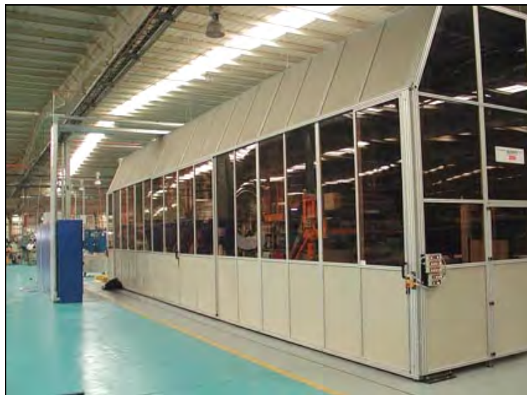
Figure 4.2 Encapsulated integrated chromium plating line [140, Atotech, 2003]
