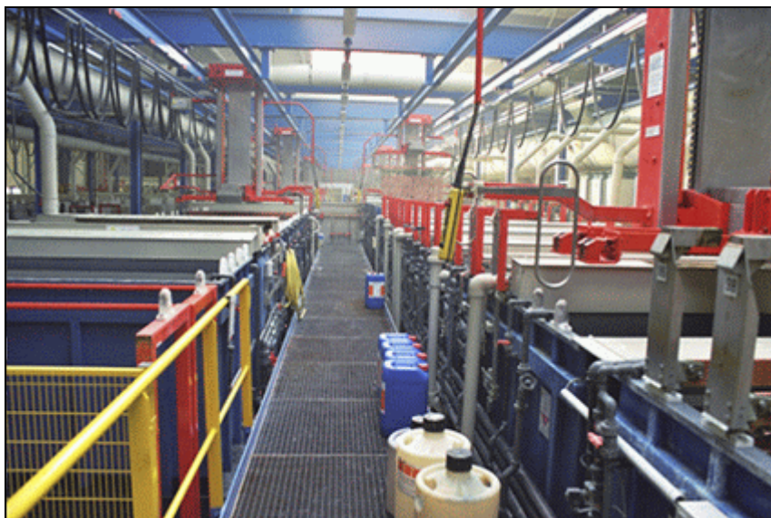
Figure 4.33: Jig line with lids on vats and air extraction Graindorge S.A. and Agence de l'eau Seine-Normandie
