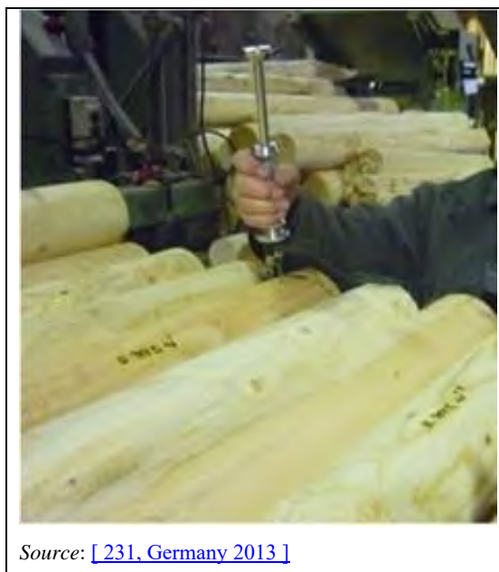
Figure 15.27: Manual wood moisture measurement
