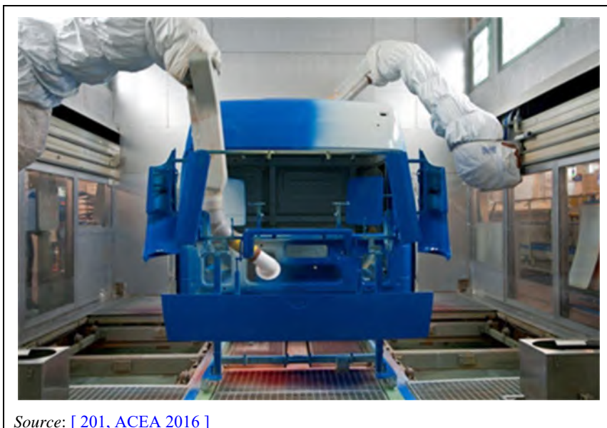
Figure 2.14: Truck cabin painting
