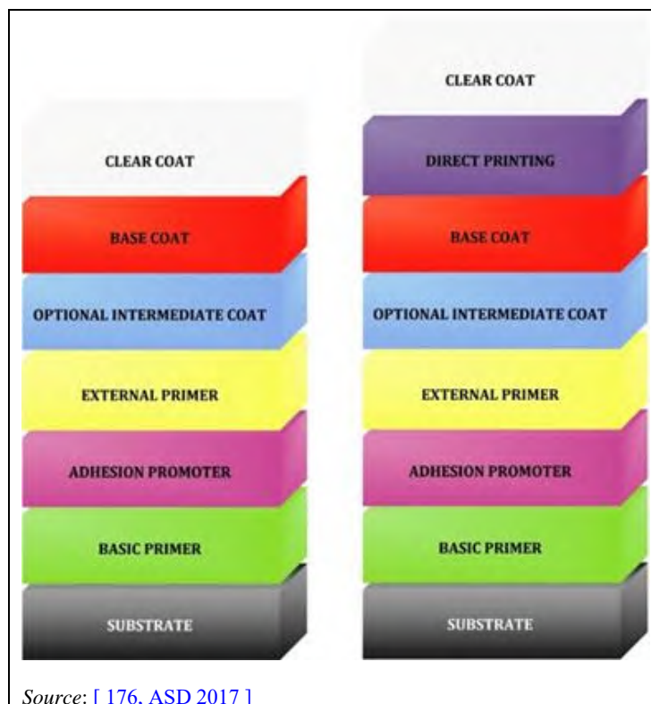
Figure 5.11: Comparison of BCCC (base coat / clear coat) system with direct printing in the BCCC system
