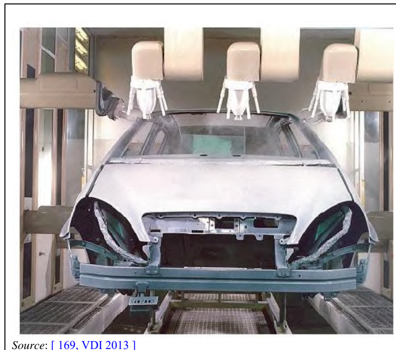
Figure 2.40: Automated paint application using painting machines
