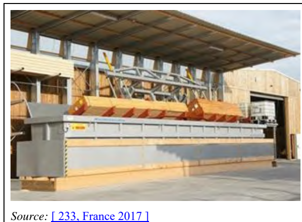
Figure 15.5: Example for brief dipping (short-term dipping / timed immersion) - tank allowing the simultaneous treatment of several batteries with the fixing done on racks next to the dipping tank
