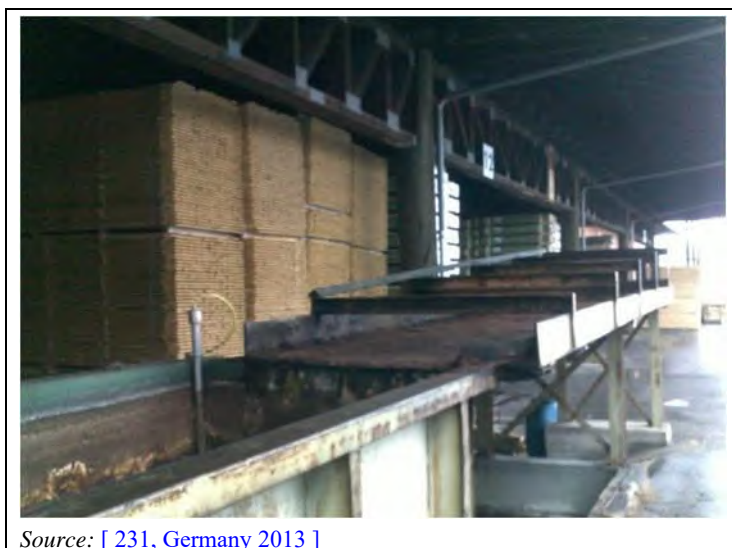
Figure 15.29: Example of a roof cover in the area of the troughs (Plant DE-4)
