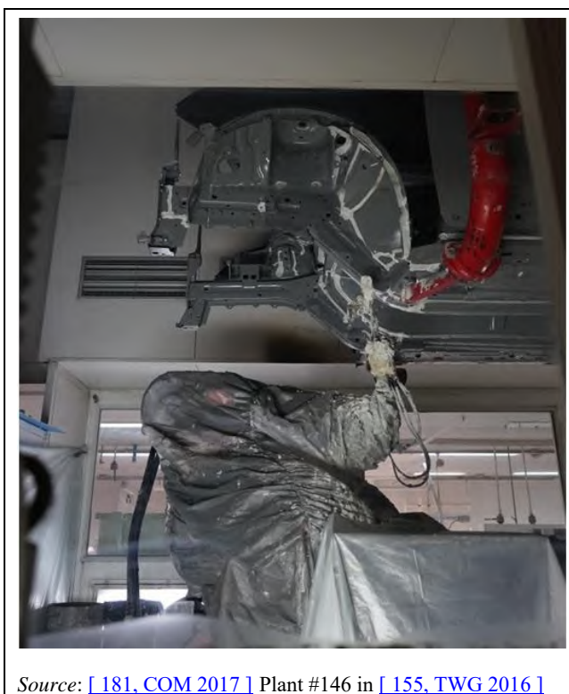
Figure 17.11: Robot applicator of sealant protected by a fabric cover
