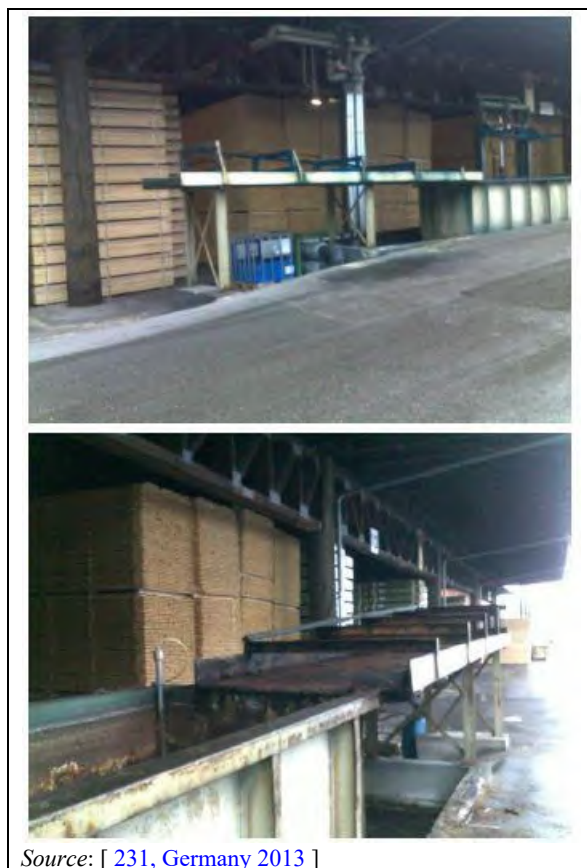
Figure 15.28: Example of a drip pad with dripping treatment solution flowing back into the treatment vessel
