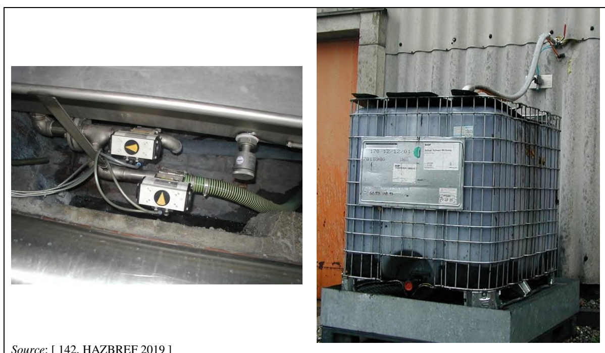
Figure 4.20: Example 2 - Automated system for the collection of spent padding liquor (left) and IBC receiving the spent padding liquor (right)
