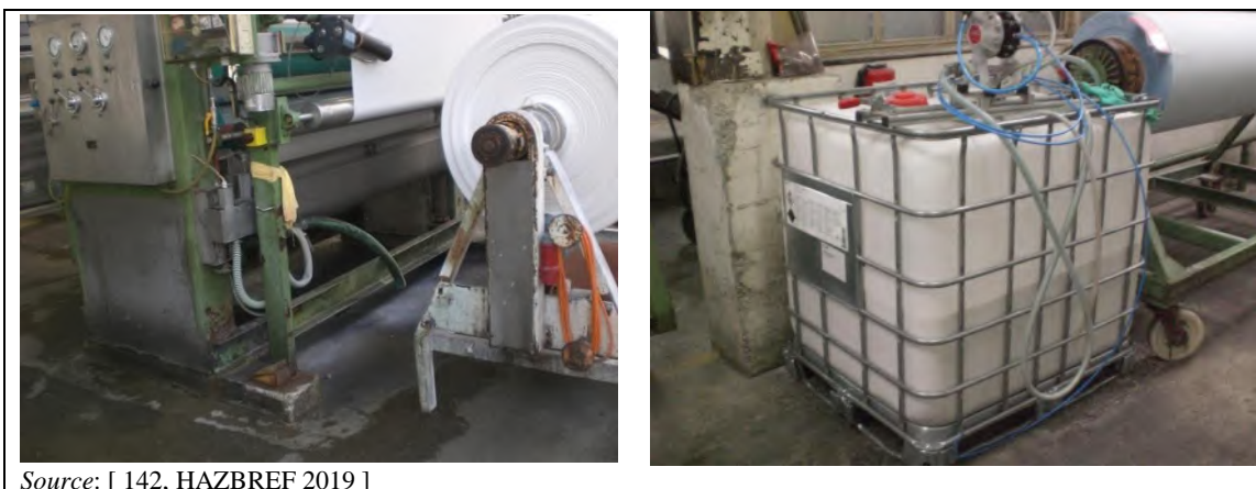
Figure 4.19: Example 1 - Padder (left) and IBC (right) equipped with a pump and pipes to manually empty the padder
