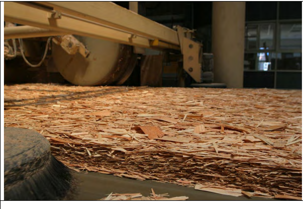
Figure 2.8: OSB mat after forming and trimming
