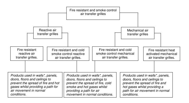
\*This includes use in the walls of fire resistant service ducts which, in normal operating conditions, permit heat release from the cables within the duct.
