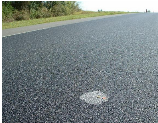
Figure C4 Satisfactory UTLAC – homogeneous texture
