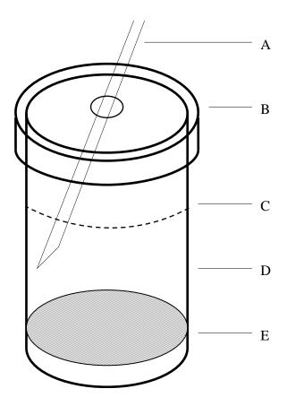
Pasteur Pipette for air supply of the overlying water glass lid to prevent emerged midges from escaping water surface layer A:
