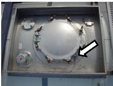
Figure 9.14 Manway hatch seal
