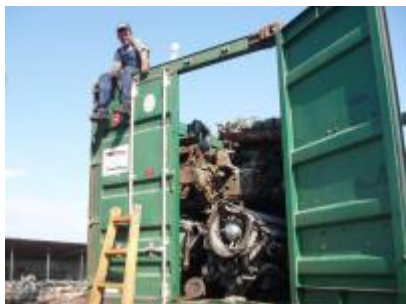
Figure 3.22 – 20-foot open top with scrap steel
