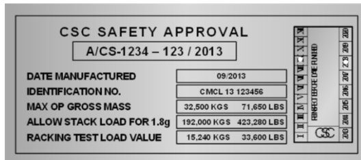
Figure 8.1 CSC safety approval plate with next examination date
