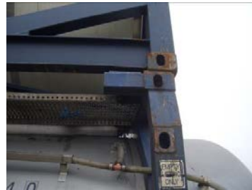
Figure 4.9 Step back with secondary side lift aperture
