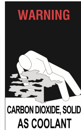
Figure 5.19 Dangerous atmosphere label
