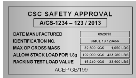
Figure 8.2 CSC safety approval plate with ACEP mark
